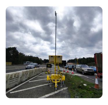
▲ Mobile VMS patented queue detection sensors communicate with each other, WAZE, and provide real-time automated advance warning to upstream VMS
