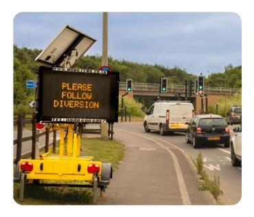
▲ Mobile VMS on the A3 diversion routes off the mainline (M25 Jn 10). The Balfour Beatty control room activated messaging on these VMS remotely, with the option to automate real-time message displays activated by changing road condition information.
