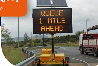
The sensor detects stopped or slow traffic in seconds, reducing the risk of rear-end collisions.
